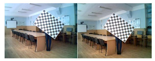
Since the required accuracy is achieved with substantial redundancy of the initial information for calibration, it was decided to record at least 10 images of the calibration pattern from different angles for each of the two channels. It is desirable to make these pictures in such a way, that the template plane is close enough to the frontal plane of the stereo pair to be calibrated.
